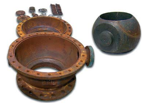
Ball valve DN 300 (12") dislocated after 10 years Service in a Chlorosilanes line inspected, maintained and released to service
